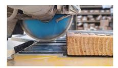
We recommend using a piece of plywood or 2x12 with a thin channel cut through it to allow the tile saw's blade to pass through but to prevent the pieces bending while cutting.
