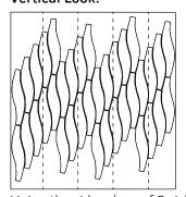
Lining the side edges of Swish parallel to walls will result in pieces being in line with each other (above and below), note that top and bottom edges of piece will not be perpendicular to the Ceiling/floor.
