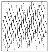
Lining the top and bottom edges of Swish perpendicular to floor/ceiling will result in pieces (above and below) angling away from eachother.
