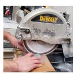
Make sure the wet saw has abundant water flow and <u>cut slowly at 30 seconds</u> <u>or more per inch</u>. Use a new piece of cardboard for cutting each tile. Keep saw table clean.
